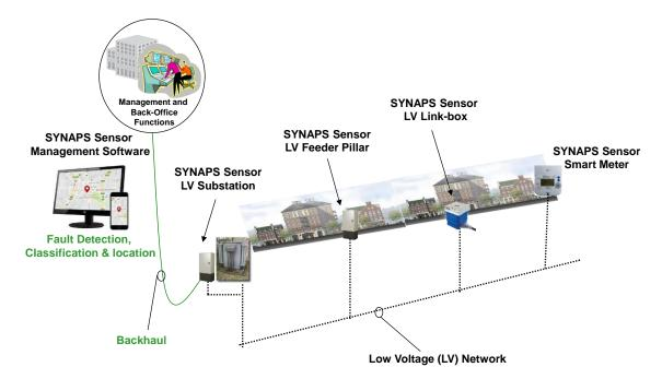
The solution consists of sensors placed in the LV substation and link boxes, or feeder pillars.
