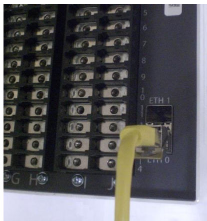
Figure 1-32 Remove communications cables (left) and SFP modules (right) BEFORE removing the relay
